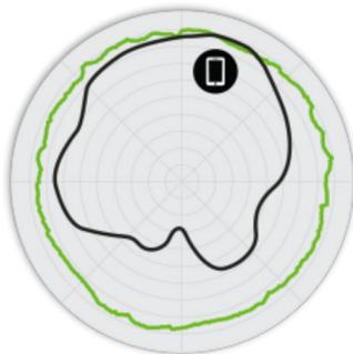
Figure 3. A750 5GHz AzimuthAntenna Patterns
