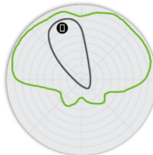
Figure 5. A750 5GHz Elevation Antenna Patterns
